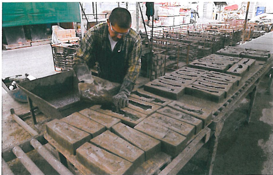
Employee pouring a concrete log.
